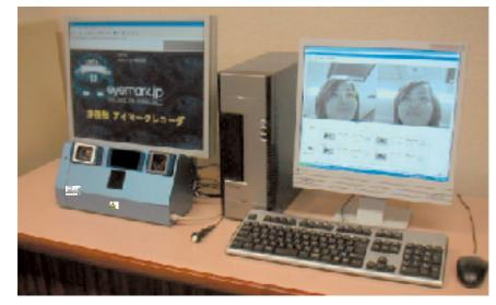
100% Contact-free, thus an examinee does not wear any special device (helmet, headband, glasses, and others) for measurements. NAC EMR-AT VOXER allows users to tack gaze position on monitor/display without any physical contact with the examinee.
