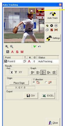
Track targets within the image. The HotShot e64's Motion Analysis Software capitalizes on MIC's expertise in high-speed image capture and image analysis, presented in an intuitive, easy-to-use software system. The software automatically tracks up to three points in the image sequence or manually tracks up to ten (10) points. The results are saved as \*.CSV files and can be exported to a variety of spreadsheet applications for further analysis.
